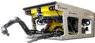
Figure 9: A ROV (Remote Operated Vehicle) System Source: ("Sub-Atlantic - Electric ROV Systems and ROV System Components", s.d.)
