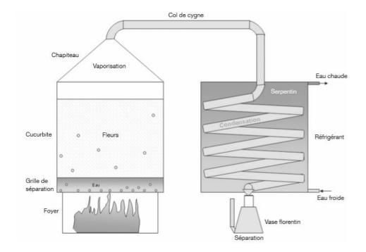
*Figure 24: An illustration of the components of a traditional steam-distillation alembic system. Retrieved from Benini et al.* (2010).
